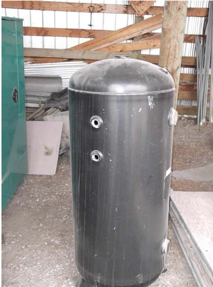
Air Compressor tank
